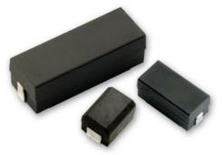
The **MILP1812**, **MIL4922** and **MIL8532** meet all Military QPL requirements, and the ruggedized molded and leaded construction is proven against MIL-STD-202 mechanical vibration, moisture resistance, and DWV testing. All "T" Level inductors are thermally shocked for 25 cycles, burned-in for 96 hours, and x-ray inspected before customer delivery.
